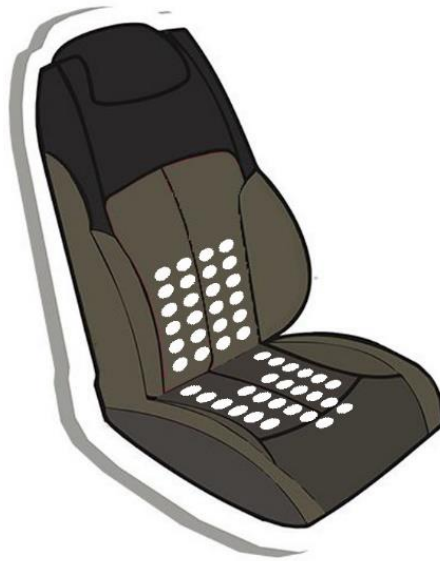
Figure 37. Illustration of the vibrotactile seat and the location of the 48 vibration motors (i.e., white circles). The motors are arranged in two matrices of 6x4 motors. One in the seat back, the other in the seat bottom.
