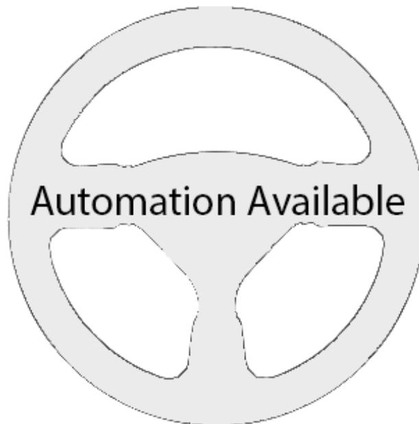
Figure 14. The icon is shown when the automation becomes available. The icon was coupled with a computer generated voice message stating “automation available”.
