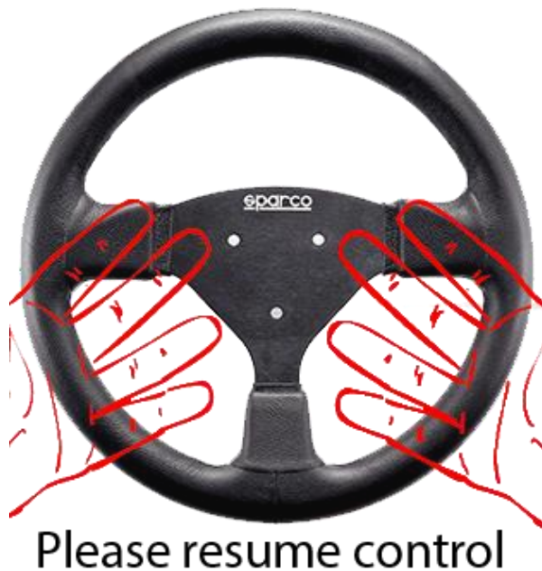
Figure 15. The take-over request icon shown on the instrument cluster. The icon was coupled with a computer generated voice message stating "please resume control".
