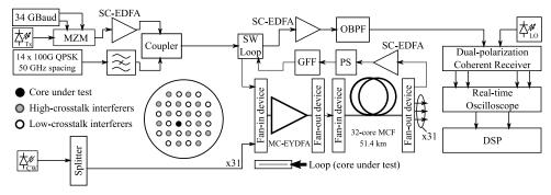
Fig. 7. Experimental setup for amplifier testing.
