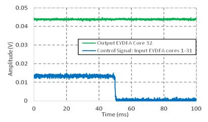
Fig. 6. Output for core 32 (green), and input signal to the reamining cores.
