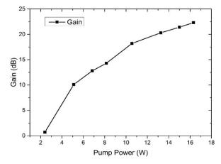
Fig. 4. Gain vs pump power for core 32.
