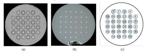
Fig. 1. Microscope image of (a) passive 32c-MCF and a core pitch matched (b) 32c-MC-EYDF, and (c) Schematic with Core indexing in 32c-MCF.
