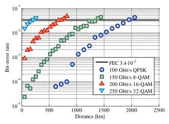
Fig. 8. BER vs distance for different m-QAM modulation formats.
