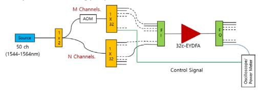
Fig. 5. Schematic setup for measuring transient performance of the 32c-EYDFA.
