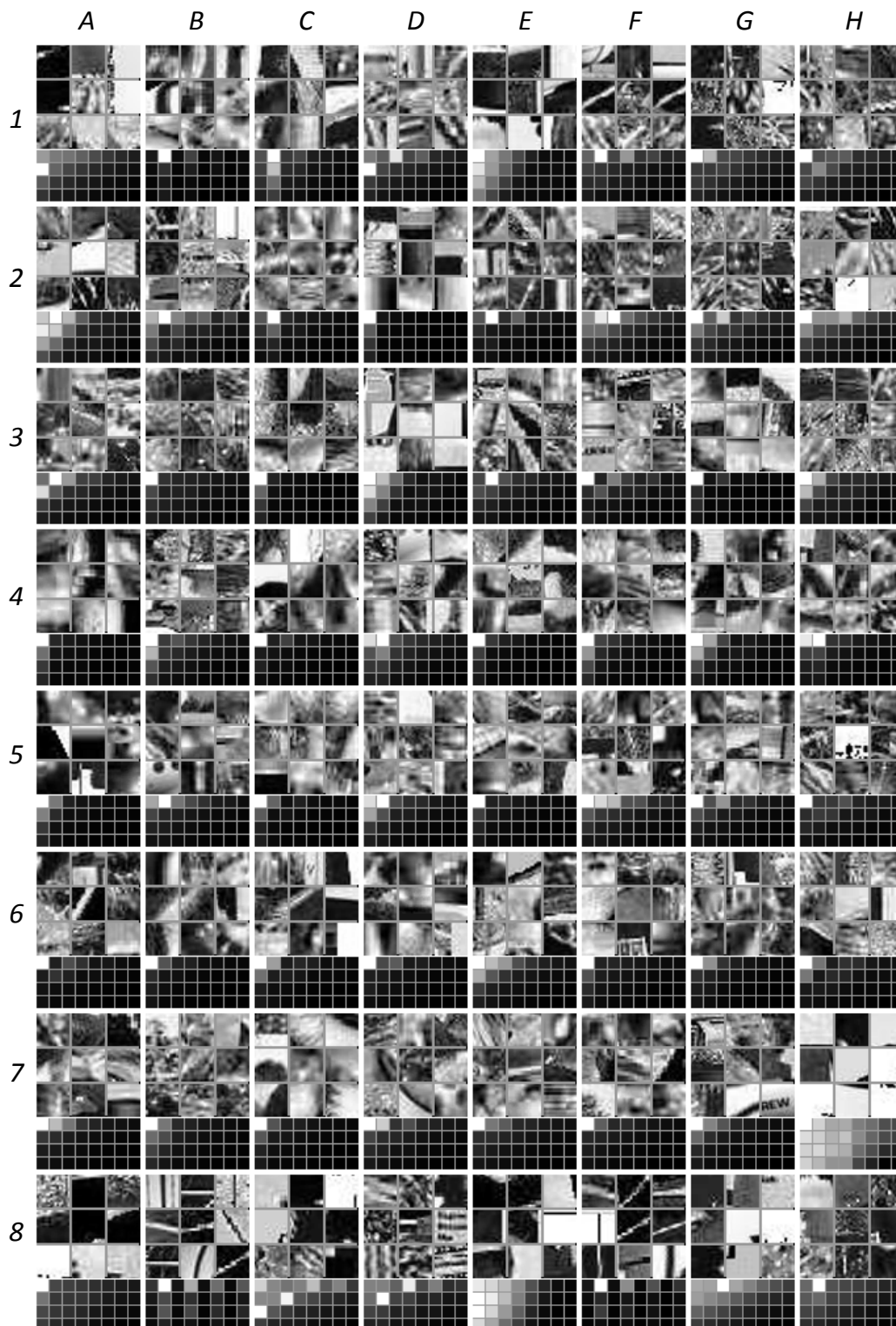
Figure 5.10: The nine closest patches to each of the learnt centroids. The three symmetry groups are present, the non-symmetric group usually captures noisy patches or translated edges (H7, H8 or D5), the symmetric group has a good response on roof edges of varying width (B1, E2 or B8) and, the composite-symmetric group which tends to highlight step and ramp edges (A4, D2 or E4). The centroids are brightness normalised for easier visualization.
