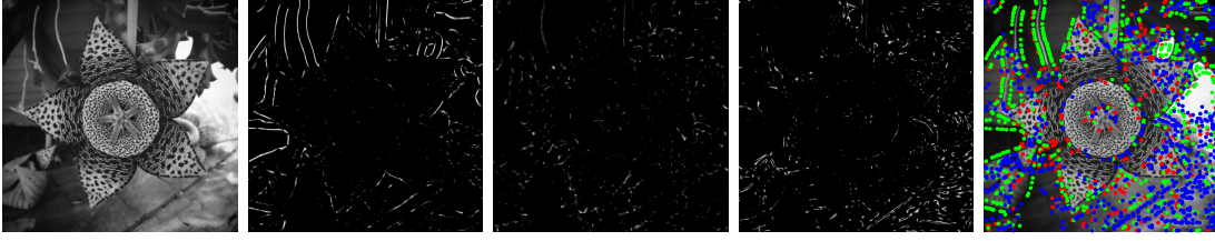
Figure 5.12: Using the learnt centroids we create feature maps D_c(x, y) (three middle images), from an original image (left). Features are detected by applying non-maxima suppression on the maps. Each of the different feature classes is a different colour on the image at the right.
