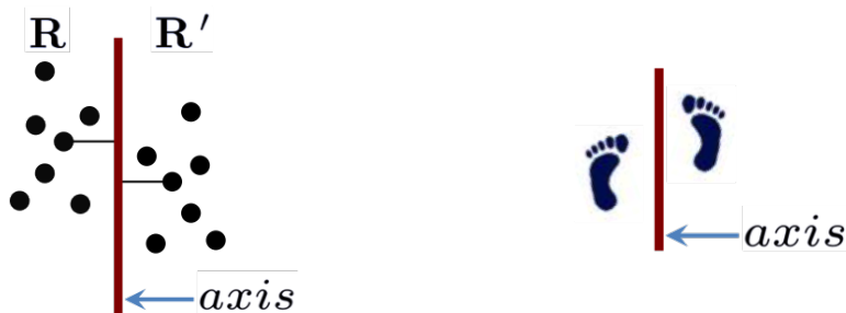
Figure 1.2: Examples of glide-reflection symmetry. A reflection plus a translation across the axis generates glide-reflection symmetric figures.
