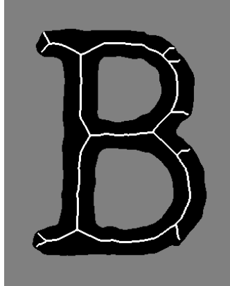
Figure 2.1: The medial axis of the letter ‘B’.
