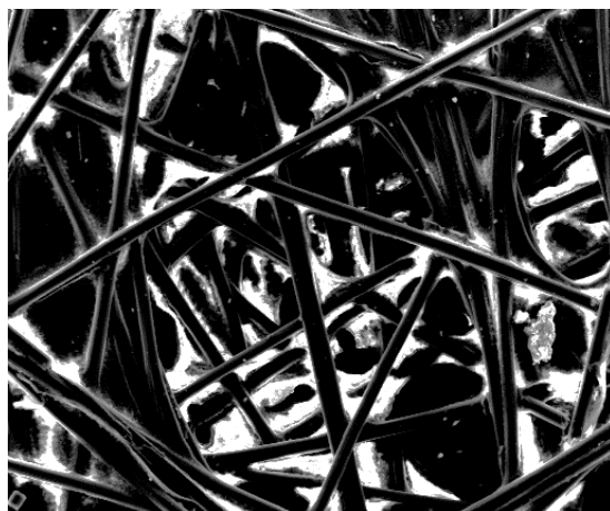
A. SEM image of carbon paper structure. The white patches show areas of fluoropolymer binder. While the black rods show the carbon fibres.
