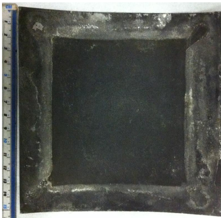
Figure 7.16 Air-electrode for the Mk II air-electrode (geometric area 150 x 150 mm, electrolyte exposed area 110 cm 2 exposed electrode area) post cycling. The central darker region shows the area exposed to electrolyte.
