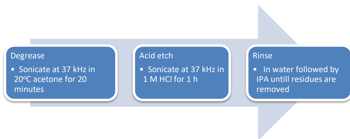
Figure 3.1 The process of pre-treatment followed for preparing metallic substrates prior to active layer application.
