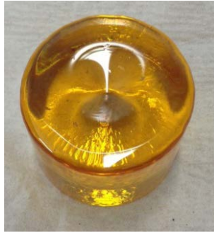
Figure 1 - Example of a glass billet casted for extrusion
