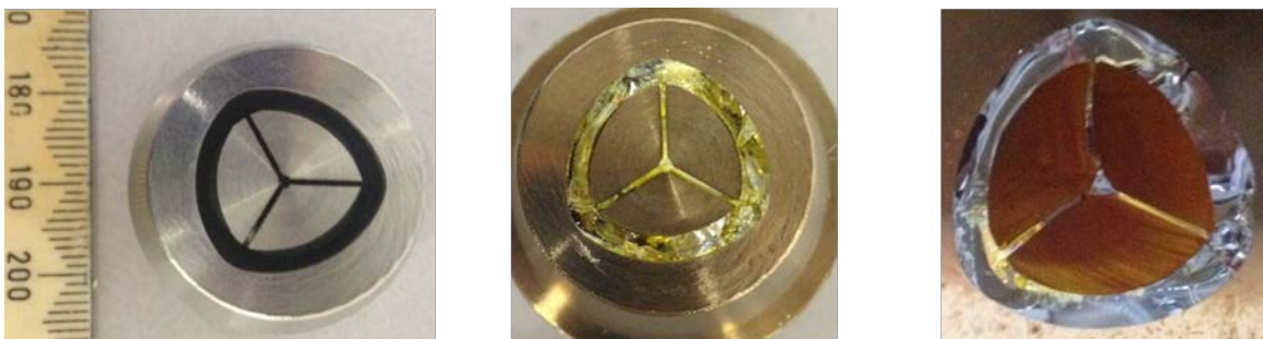
Figure 4 – (a) Extrusion die for suspended core preform; (b) Extrusion die after extrusion run; (c) Cross-section of extruded preform
