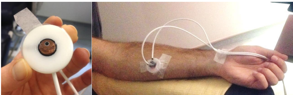
Figure 3.4 The combined LDF and WLS probe inserted into a heating disc (left) and attached to the skin (right).
