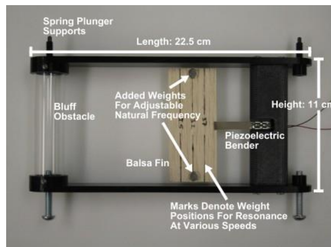
Figure 2.13: Schematic of the cantilevered piezoelectric beam. Reprinted from [85].
