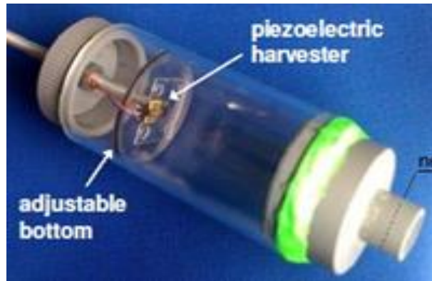
Figure 2.25: Helmholtz resonator with the piezoelectric cantilever harvester. Reprinted from [117].
