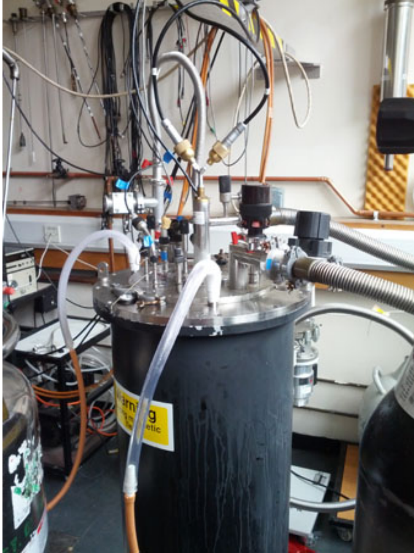
Figure 3.22: The liquid helium cryostat used for low temperature measurements. Temperatures of between 300K and 4.2K are achieved via the combination of the evaporation of liquid helium and a resistive heater in the sample space. Also included is a superconducting magnet capable of 10T in steps of 0.1 gauss.
