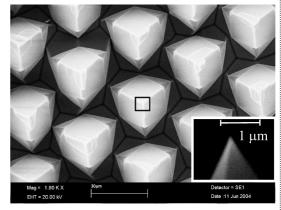
Figure: SEM image showing an array of microstructured pyramidal superstructures. The inset photo shows a high magnification side image of the tip.
