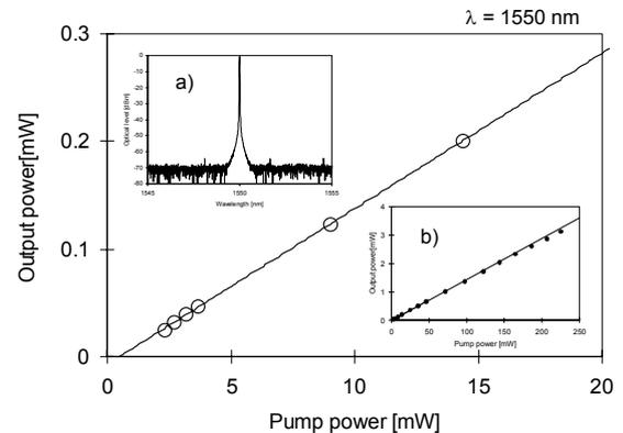
Fig.6 Output characteristics of the EDHFRL at 1550 nm near the threshold. Inset a) shows the optical spectrum (pump power  $\sim 200\text{mW}$ ) and b) the output characteristics over the full range of pump power.
