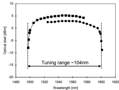
Fig.7 Output power as a function of emission wavelength of the EDHFRL at a maximum pump power. (squares: using Filter1, circles: using Filter 2).
