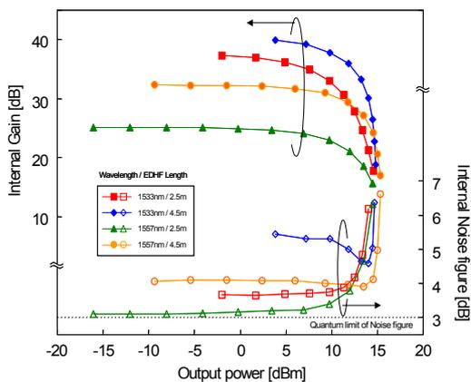
Fig.9 Gain saturation and noise figure as a function of output power for various fiber lengths.
