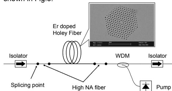
Fig.3: Schematic of the EDHFA gain-block (reverse pump configuration). Inset shows the SEM picture of the EDHF core.
