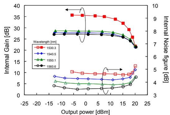
Fig.11 Internal gain saturation and noise figure as a function of output power for various wavelengths.
