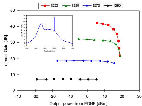
Fig.4 Gain saturation characteristics of the EDHFA at various wavelengths. Inset shows the ASE spectrum with small signal gain conditions at 1560 nm.
