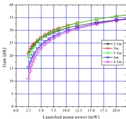
Fig.10 The gain efficiency curves for different fiber lengths. Maximum gain-efficiency = 8.6dB/mW.
