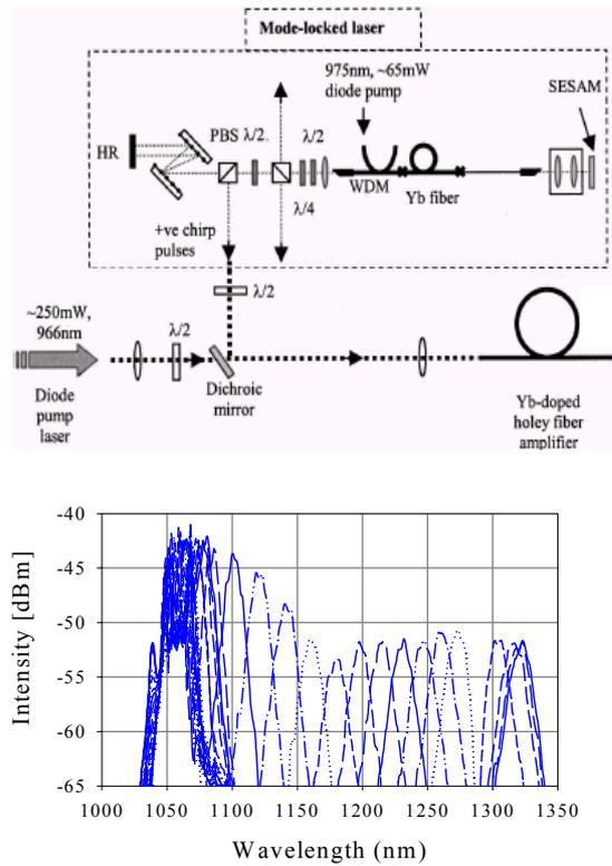
Fig.2 (a) Schematic of system. (b) The spectra of continuously-tunable Raman solitons at the YDHF output for pump-powers in the range 0-200mW.
