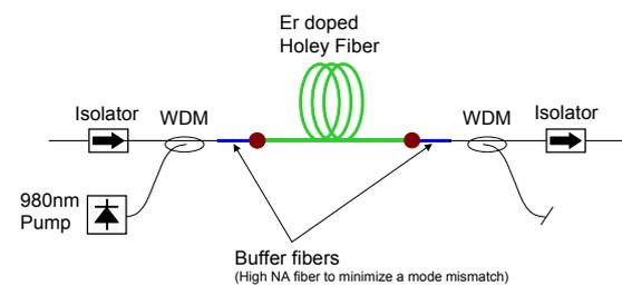
Fig.8 Schematic diagram of the low noise EDHFA.
