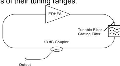
Fig.5 Schematic diagram of the EDHFRL.
