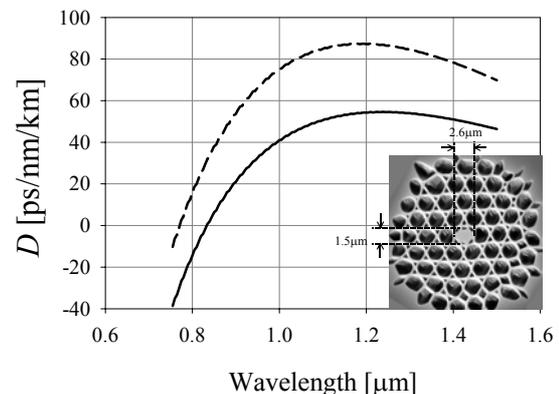
Fig.1 The predicted dispersion for the two birefringence axes of the YDHF (SEM shown inset).
