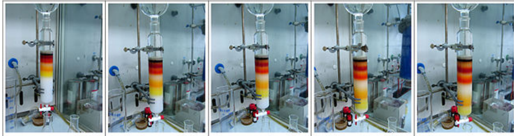
Figure 5.2: Examples of a Column Chromatography Experiment (Zlatich, 2013): These five photos are taken at different times of a column chromatography experiments (starting from left to right). Substances in the mixture have different colours. They are poured into the column from the top at the beginning. After some time, the substances slowly separate into different layers in the column.
