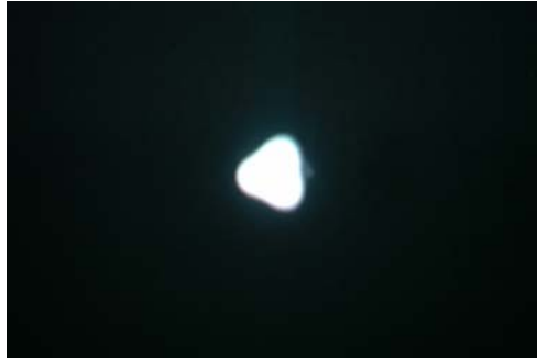
Fig. 2 IR image of the near-field pattern of the connectorized Bi-HF.
