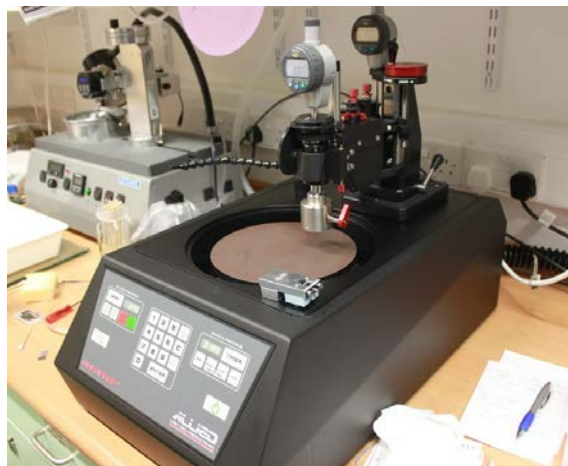
Figure 2.26 – Allied High Tech Products Inc Multiprep™ lapping and chemical-mechanical polishing equipment.
