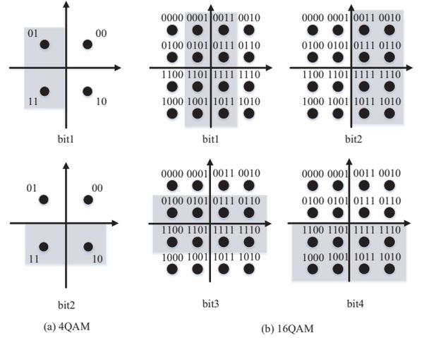
**FIGURE 1.** The subset partitioning for each of the two or four bit position of (a) 4QAM or (b) 16QAM coherent state constellations. The numbers above the constellations point represent the binary information bit. The shaded regions correspond to the decision regions for  $x_i = 1$  and the unshaded region correspond to  $x_i = 0$ .
