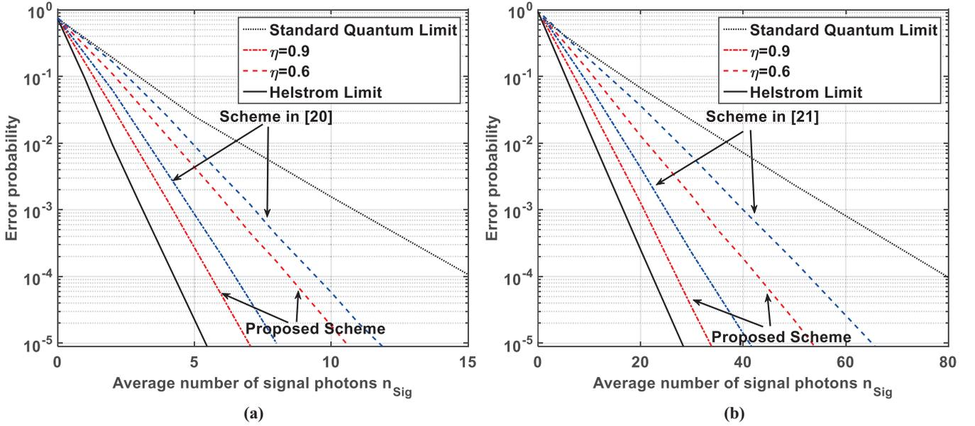
FIGURE 9. Error probability of the iterative receiver and the conventional non-iterative receiver under different quantum efficiency for (a) 4QAM (b) 16QAM.
