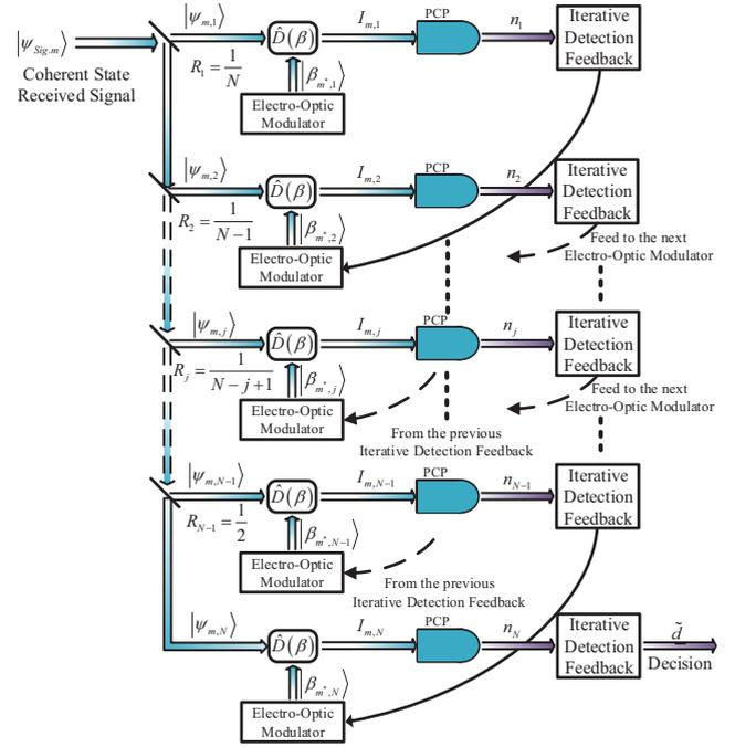
**FIGURE 4.** The schematic of the soft iterative quantum receiver. The diagonal lines at the input represent the beam splitters.  $\hat{D}(\beta)$  is the displacement operator and the PCP represents the photon-counting process using the PNRD.
