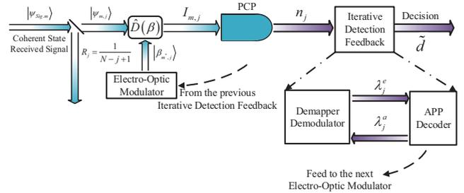
**FIGURE 3.** The schematic of the soft iterative quantum receiver for  $j$ th measurement approach. The diagonal lines at the input represent the beam splitters,  $\hat{D}(\beta)$  is the displacement operate and the PCP represents the photon-counting process using the PNRD. The result of detection  $n_j$  is sent to iterative detection feedback for iterative demapping and decoding. A final decision  $\tilde{d}$  is performed considering the outcomes obtained on the  $N$  different parts.
