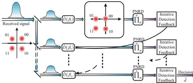
**FIGURE 2.** The receiver splits the received 4QAM signal into  $N$  parts. Quantum state after splitting is displaced by  $\hat{D}(\beta_j)$  and then measured by a PNRD. Via iteration and feedback control, the value of displacement  $\hat{D}(\beta_j)$  in each part depends on the output of iterative detection feedback block.
