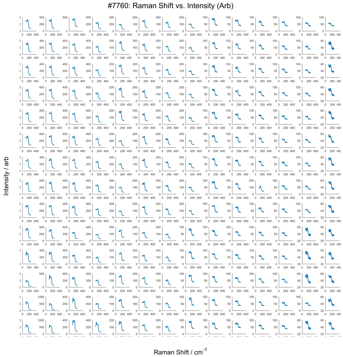
Figure B.9: Raman spectra of N-GST sample #7760, annealed in vacuo at 300 °C for 20 min.
