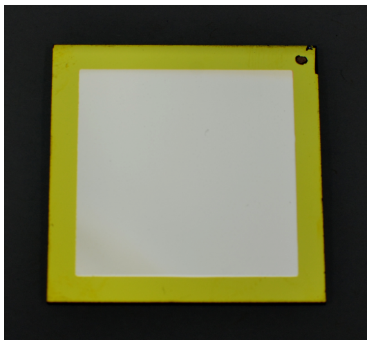
Figure 5.10: Photograph of an N-GST library annealed at 300 °C for 20 min (#7760) with compositional points shown in Figure 5.3.
