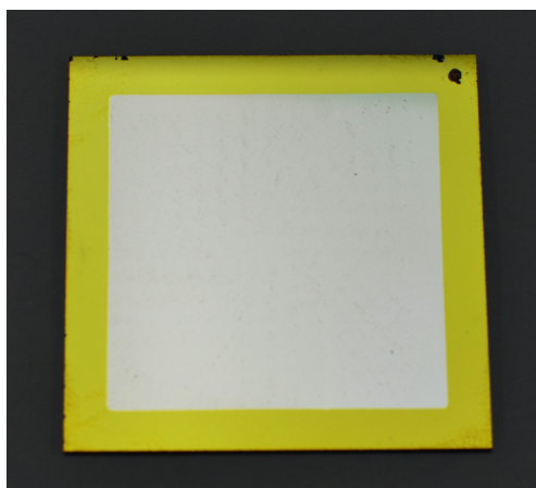
Figure 5.4: Photograph of an as-deposited N-GST library (#7754) with compositional points shown in Figure 5.3.
