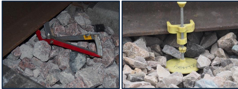
Figure 2.3 Examples of void meters installed on the track.
