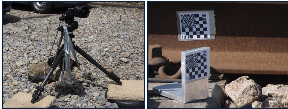
Figure 2.6 Photographs of (a) a high-speed camera and (b) calibration targets for digital image correlation, (Watson, 2016).
