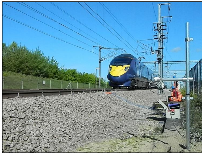
Figure 3.7 Photograph of the Crissmill plain line site instrumented during combined track vibration and aerodynamic measurements (Watson, 2016).
