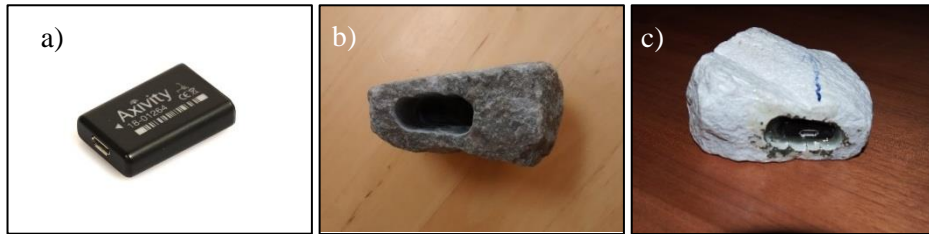
Figure C 1 (a) AXIVITY AX3, (b) Ballast grain with slot for sensor (c) Instrumented grain ready for use.
