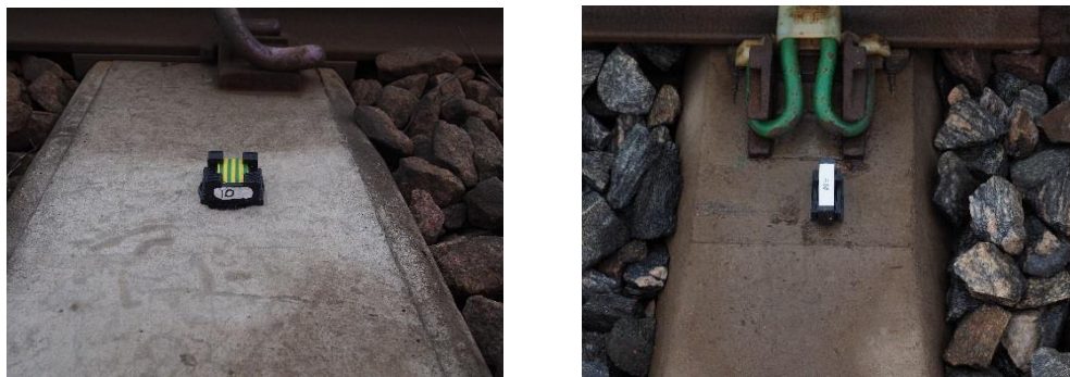
Figure 4.13 Photographs of (a) AX3 and (b) X16 accelerometers deployed on track.
