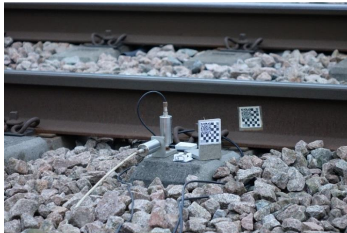
Figure 4.8 Photographs of geophones, MEMS accelerometers and targets for DIC mounted on a sleeper end (Watson, 2016).
