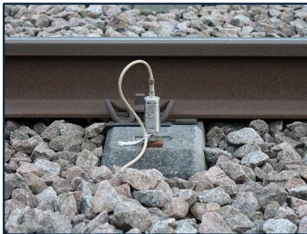
Figure 2.4 Photograph of a geophone on a sleeper end (Watson, 2016).
