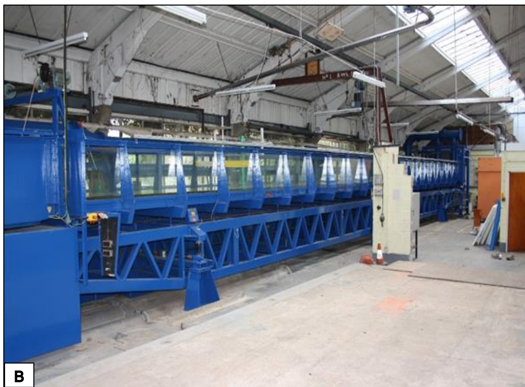
Figure 3.1. Recirculating flumes at the ICER facility used in this research: A) 12.0 m long indoor flume, B) 21.4 m long indoor flume.
