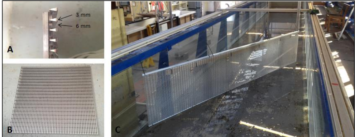
Figure 6.2. Details of wedge-wire panels used throughout the study. A) Close-up of the side of a single panel illustrating the 3 mm profile bar width and 6 mm spacing; B) Plan view of a single 50 cm x 50 cm panel when profile bars are vertically oriented; C) wedge-wire screen (horizontal profile bar orientation) made up of a frame with five slotted panels in a large recirculating flume to create the plan view as shown in Fig. 6.1. The bypass channel was located at the far right.
