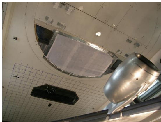
Figure 137 - Images showing acoustic array mounted in the ceiling of the Filton wind tunnel test section.
