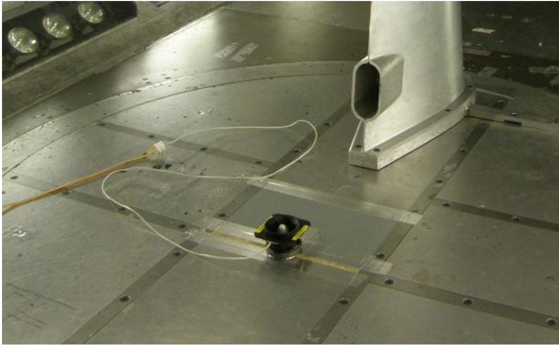
Figure 136 – Noise Source used for testing acoustic array.
