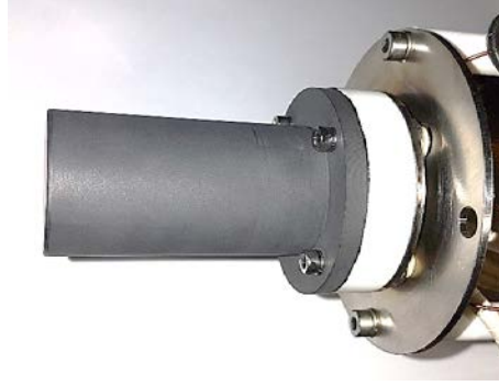
Figure 1. Mounted second-generation LaB 6 heaterless hollow cathode
