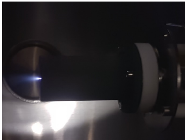
Figure 12. HHC Keeper only discharge, 2 nd configuration, \dot{m} = 1.75 sccm, I_k = 2 A
