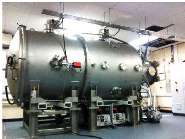
Figure 1: David Fearn Electric Propulsion laboratory vacuum chamber at University of Southampton
