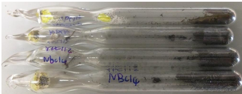
Figure 2.2 The product of \text{NbCl}_5 reduction in sealed tubes at 350^\circ\text{C} . The black needle crystals and brown powder at the right side are \text{NbCl}_4 identified via PXRD analysis and from IR spectroscopy. The white powder assumed to be \text{Nb}_2\text{O}_5 and the yellow solid is \text{NbCl}_5 .
