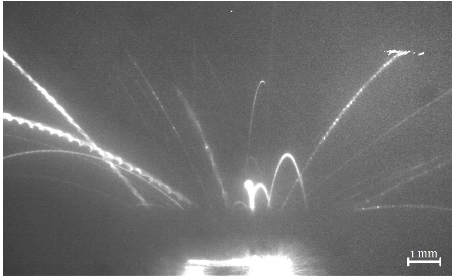
FIGURE 5.7: A wide illumination area of particle release at high vacuum, 10^{-6} mbar, with path arcs that allow the velocity to be calculated. The spiral path is assumed to be due to the irregular shape of particle clusters. This particle release was at 10 watts of driving power and the velocities are estimated to be 0.3 \pm 0.1 m/s
