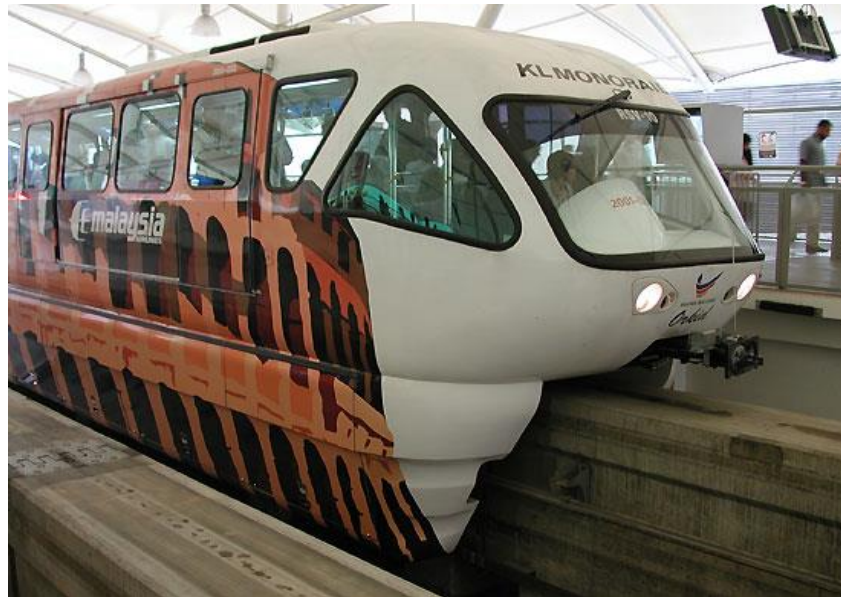
Figure 4.42 The Roman Coliseum is featured on this Malaysia Airline-sponsored train. The coupler allows train link-ups for extended trains or in rare circumstances, the towing of inoperable trains.
