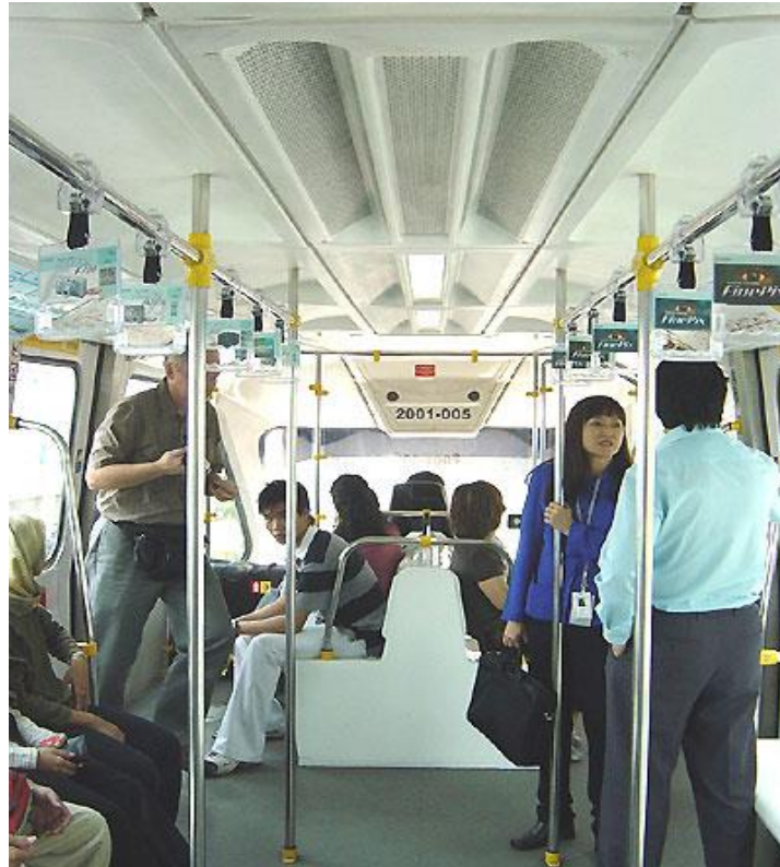
Figure 4.41 The center seat also serves as a cover of the load-bearing wheels.
