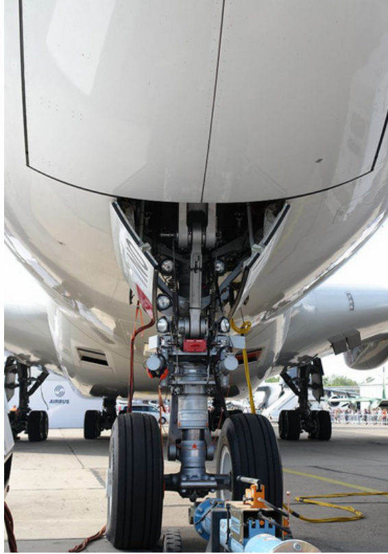
Figure 2.2: Image of the Airbus A380 nose landing gear with gear deployed, front doors closed and rear doors open; reproduced from [78].
