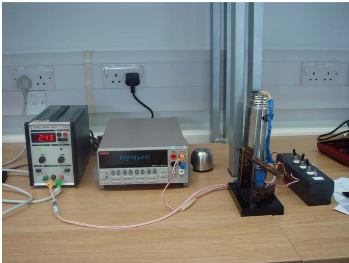
Figure 2-12 – A photograph of the custom built 2 point probe Seebeck measurement unit used in this work. Photograph courtesy of Elena Koukharenko.
