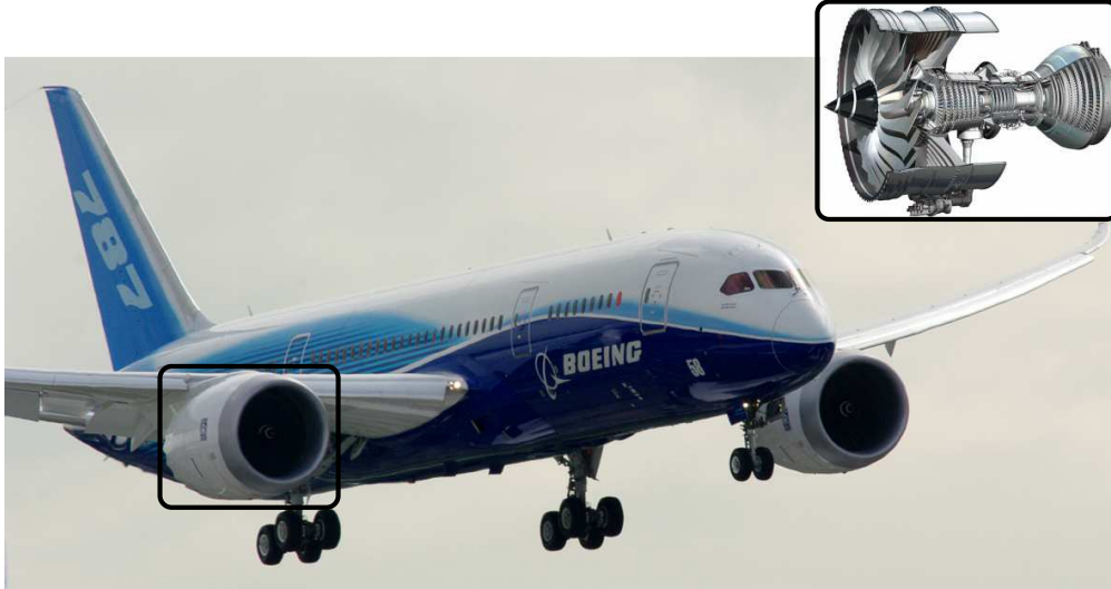
Figure 1.1: Rolls-Royce Trent 1000 engine on Boeing 787.
