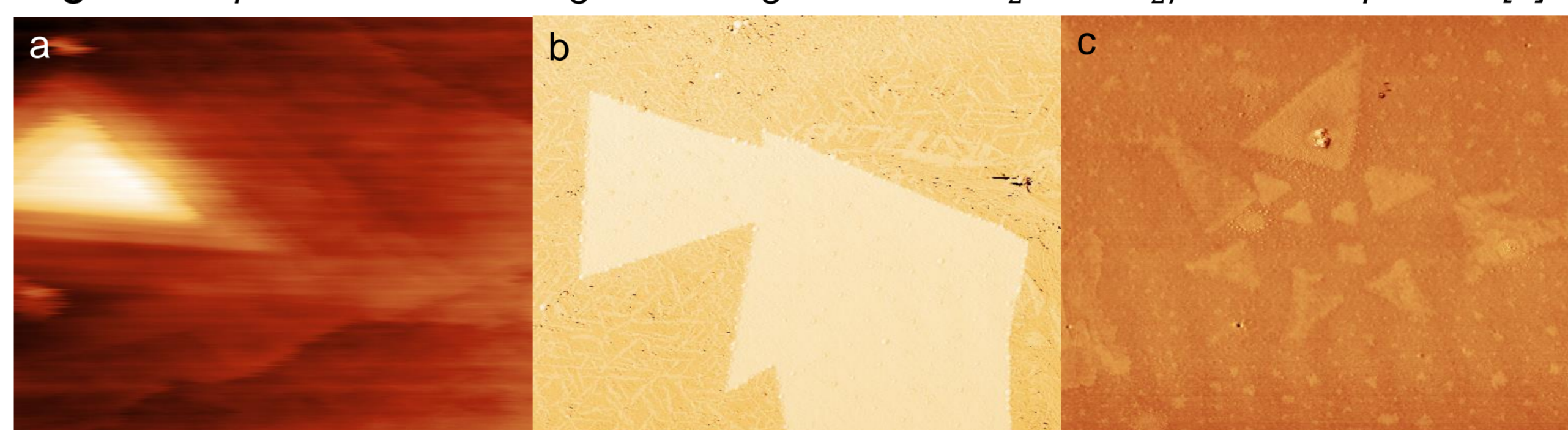
Figure 5: (a-c) Tapping-mode AFM images show triangular-faceted crystals grown by our technique. Figure 5a shows layer-by-layer stacking of crystals. Figures 5b and 5c show flakes with heights ~7.0-28.0 Å, 1-4L.
