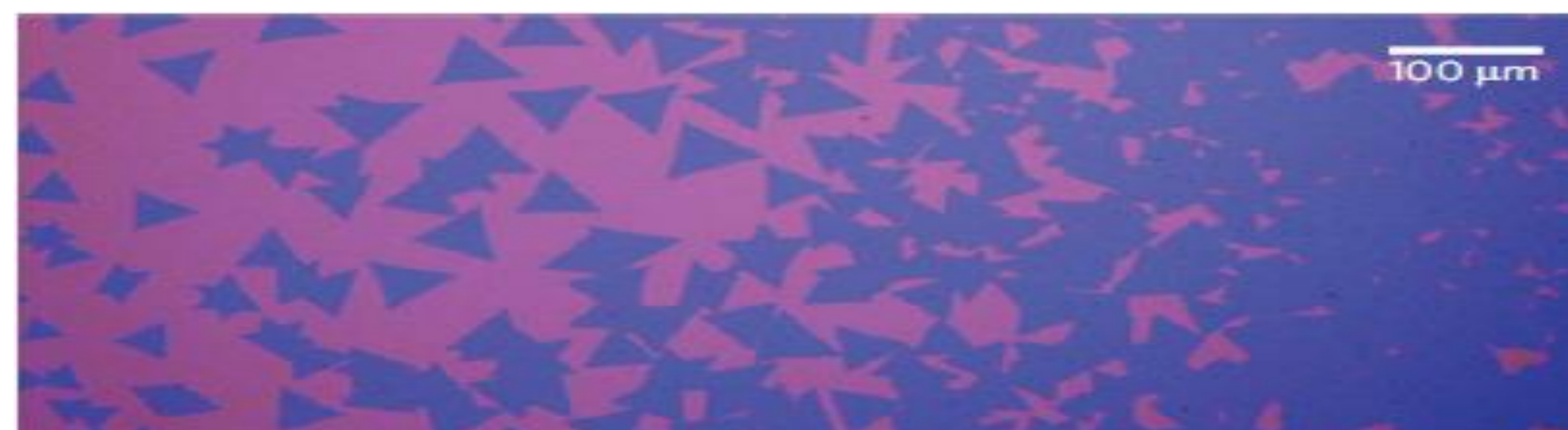
Figure 4: Optical reflection image of CVD growth of MoS 2 on SiO 2 /Si for comparison [2].
