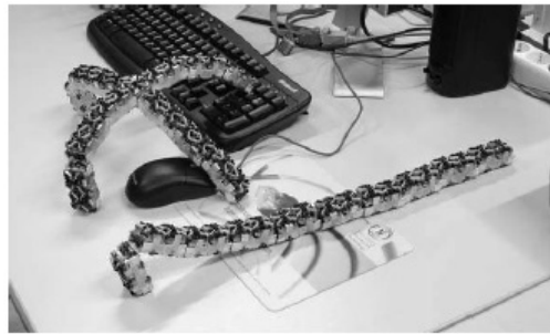
Figure 2.9: The concept of an assembled heterogeneous swarm robots from the Symbrion and Replicator projects to find power sources at other locations (Kornienko et al., 2007).
