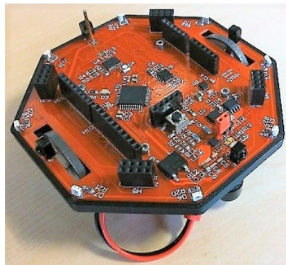
Figure 6.6: The basic OctBot, an octagonal low cost platform to aid swarm robotics research.
