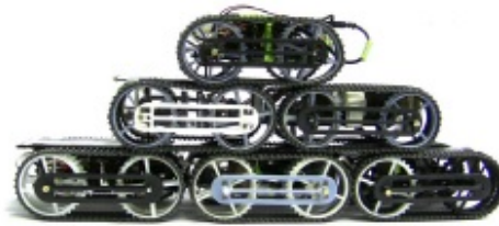
Figure 2.11: A pyramid structure formed by assembled mobile robots inspired by an ant colony to reach a higher location (Cucu et al., 2015). Robots can climb over other robots and construct a pyramid structure, whereby the above layers contain fewer robots than the ones below, so as to maintain the structural stability.
