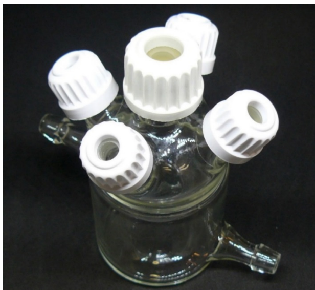
Figure 2.8. The jacketed glass cell used for the electrochemical experiments in this work; five-neck cell. The glass cells can be connected to a thermostatically controlled water bath using rubber tubes.
