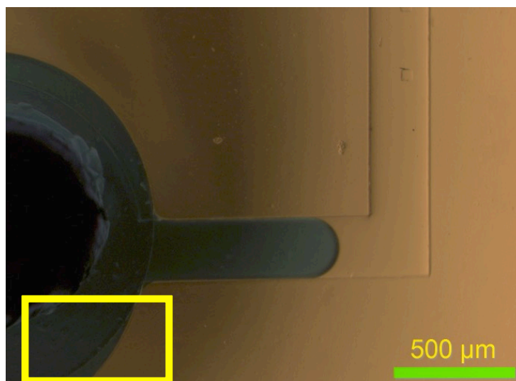
Figure 3-22: Liquid leaking after air has compromised the PDMS:PMMA seal. Scale bar = 500 \mu\text{m} .
