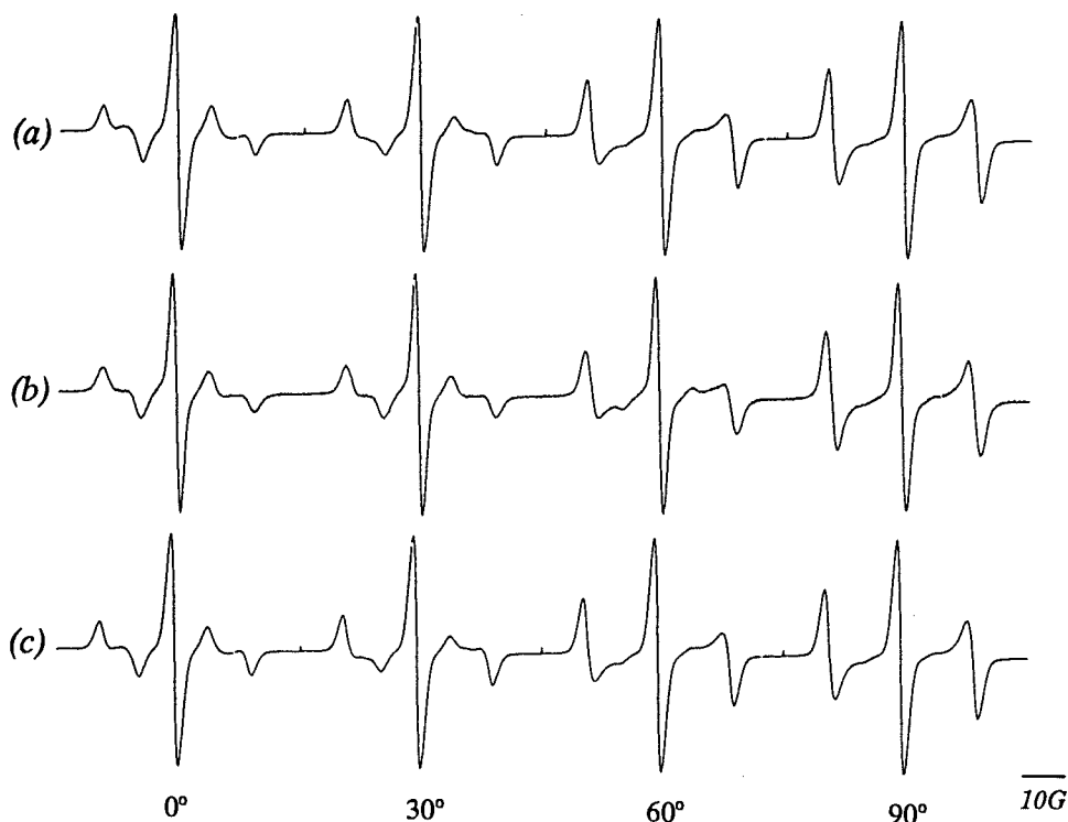
Figure 18 The spectra calculated using values of (a) a_2=1.6 and (c) a_2=1.4 in the model expression p(\cos\theta_i)=\exp(a_2 P_2(\cos\theta_i)) . The corresponding experimental spectra are shown in (b).
