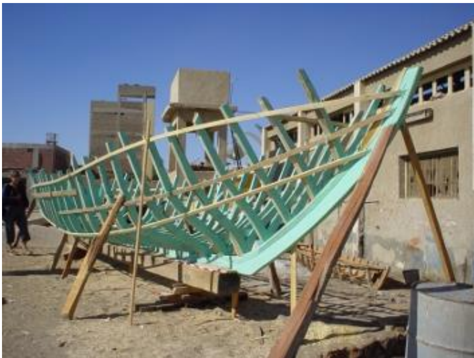
Figure 6 Photograph of a frame-first boat under construction in a traditional yard in Egypt. The framework has been erected prior to the outside planking which will be fixed to it. (Photograph Julian Whitewright)
