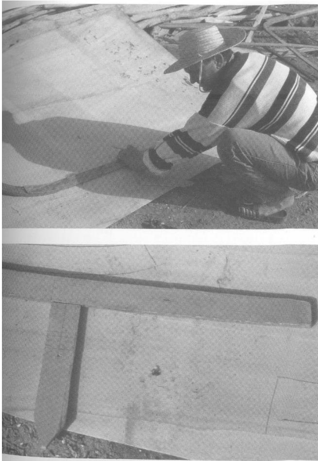
Figure 109 Tunisian boatbuilder of the late 20 th century drawing the shapes of the frames using a template of the master mould and a rising staff. By arranging both elements, the rising and narrowing of each frame can be adjusted. (Rieth, E., 2016. Navires et Construction Navale au Moyen Age , p.257)
