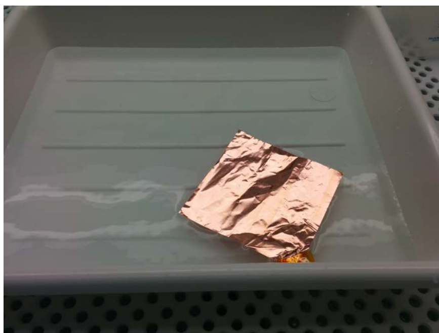
Figure 3.3: Photograph image of graphene/copper stack floating on the ammonium persulphate etchant solution
