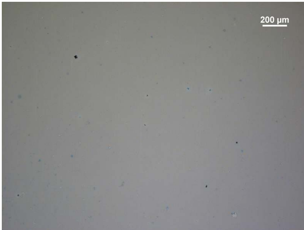
Figure 3.4: Image of large scale transfer of graphene with minimal cracks, wrinkles and residue on the surface
