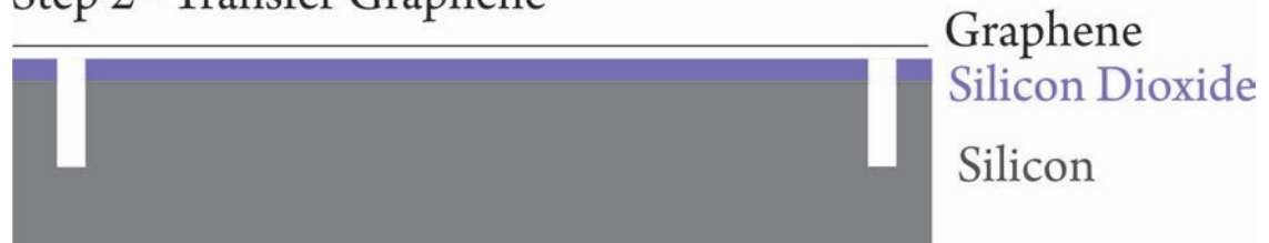
Figure 5.9: Schematic diagram to show the graphene after the transfer on the target substrate. The graphene is shown to suspend across the alignment marks in the diagram but will be broken and pull to the inside of the alignment marks for the actual transfer. If the graphene was suspended across the alignment it would cause issues with the e-beam system since a SEM is used to detect the height change in a sample from the contrast of the edges. A suspended graphene layer would prevent this.
