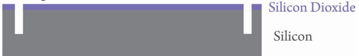
Figure 5.8: Schematic diagram of step 1 showing the oxidation of the wafer and etch of the alignment marks into the wafer
