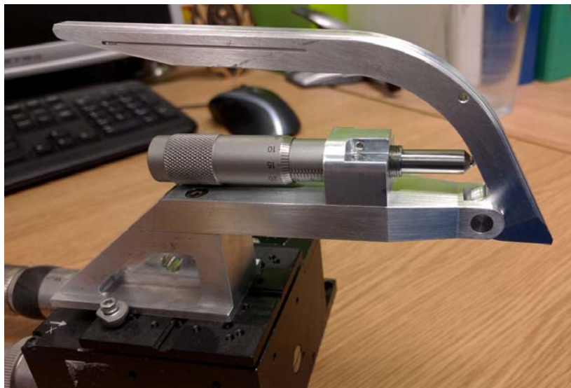
Figure 3.13 machined aluminium fibre arms.
