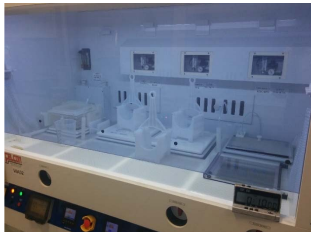
Figure 3.6 A typical wet bench with four etch baths containing (from left to right) orthophosphoric ( \text{H}_3\text{PO}_4 ) acid, RCA tanks one and two, and a KOH tank. There is also a rinse dump tank toward the front.
