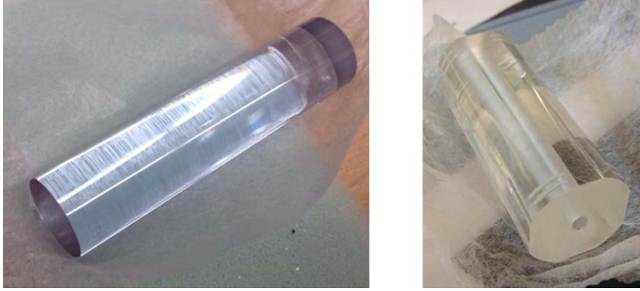
Figure 4.8: Processed doped glass (left) and undoped glass (right).
