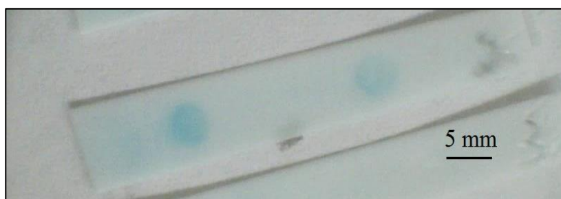
Figure 7.11 Image showing the result of the implementation of sandwich CRP ELISA on nitrocellulose membrane with a sample concentration of 90 ng/mL.
