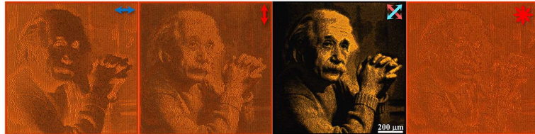
FIG. 5. The polarization sensitive Einstein's portrait imprinted in a-Si:H film by femtosecond laser nanostructuring. Arrows indicate the polarization states used for the optical transmission imaging. (Multimedia view) [URL: http://dx.doi.org/10.1063/1.4919538.1 ]
