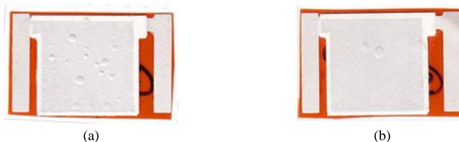
Figure 7-6: Shape deformation of the devices after applying CIP at 166 MPa for the devices protected by (a) PVC film and (b) latex bag
