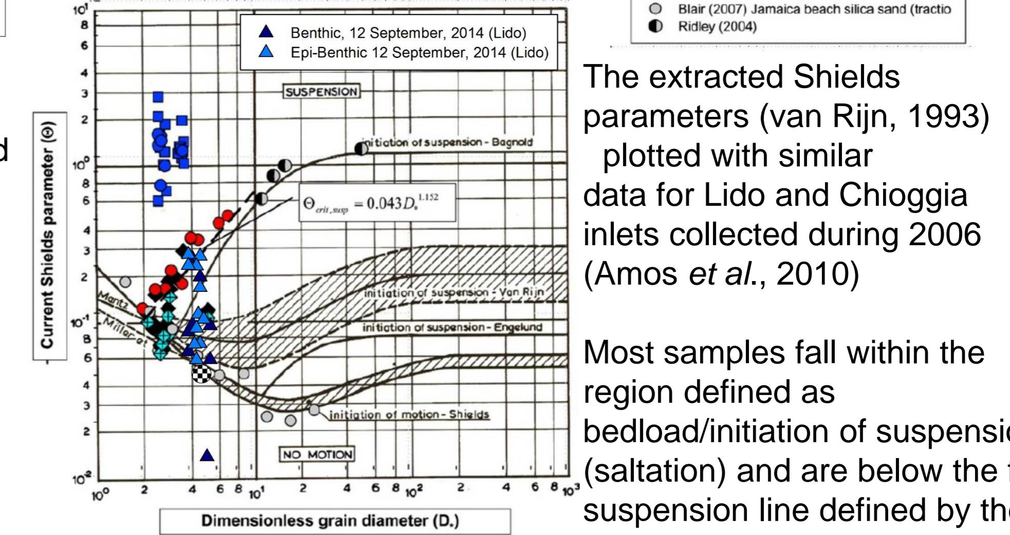
The extracted Shields parameters (van Rijn, 1993) plotted with similar data for Lido and Chioggia inlets collected during 2006 (Amos *et al.*, 2010).
