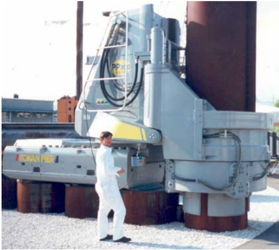
a) A 300 tonne press-in piler for installing 1000-1200 mm diameter steel tubular piles
