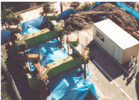
e) Aerial view of load test arrangement
