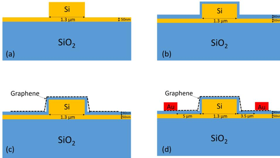
Fig. 6. Schematic cross-section of the graphene mid-IR detector.
