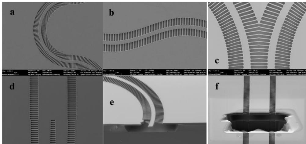
Fig. 1. SEM image of a) the 90° bend b) the s-bend c) waveguides converging towards the MMI input section and d) input section half of the MMI (top views). e) A cleaved facet of a 90° bend with the BOX locally removed, with a few destroyed silicon strips due to the cleaving. f) Under-etched multimode region of the MMI after FIB cut, with no appreciable deformation of the suspended structure [28]
