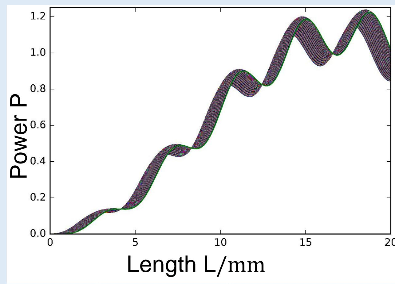
Top waveguide: points at which power does not depend on device length.
