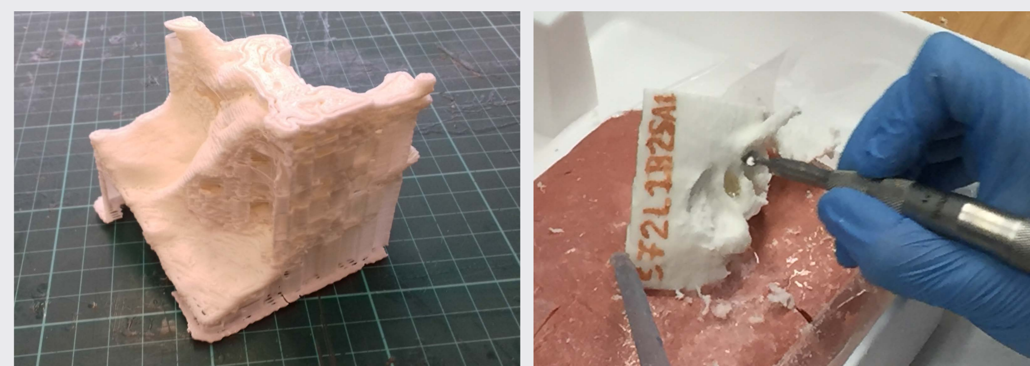
Figure 2: Left: Printed bone with support material coming off the printer. Right: Drilling of the bones for evaluation.
