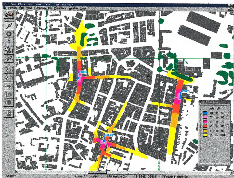
Figure 1.4: Close-up of the pathloss plot of the microcells. The grey areas are buildings, the white areas are open spaces and the green areas are vegetation.
