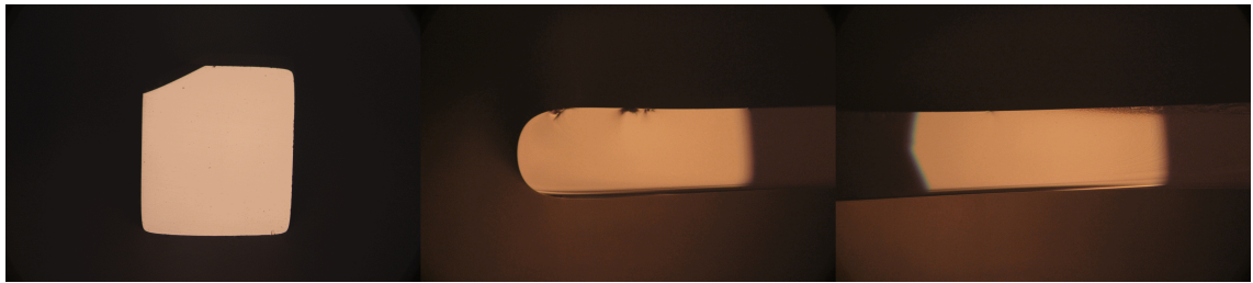
Figure 4.21: Captured images of the cleaved Nd:Phosphate draws. The full cross section of the planar structure proved too large to capture under 10x magnification. An edge and central region are shown instead
