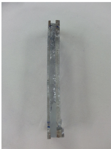
Figure 4.16: The three-layer fused phosphate glass preform
