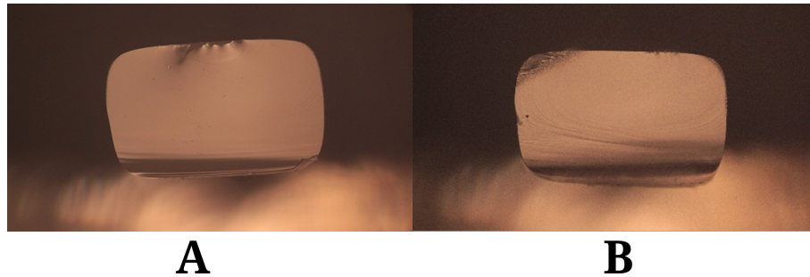
Figure 4.11: Cleaved faces of the bonded fibre cane at 10x magnification. A) A face showing a perfectly clear interface, and B) A small air gap is visible on the left-hand side
