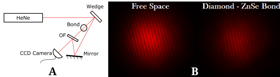
Figure 6.19: A) HeNe interferometer setup for inspecting bond interface optical distortions. One path travels through the bond before recombining with the freespace beam reflected off an Optical Flat (OF), and B) Interference patterns with both beams in free space travel and with one beam passing through the bonded composite
