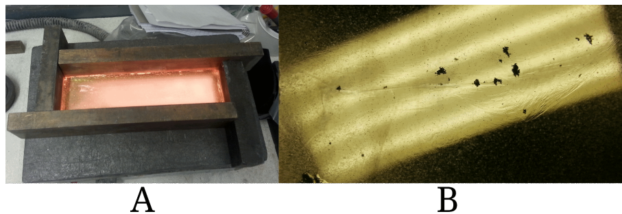
Figure 4.15: A) The custom glass melt cooling, and B) A backlit view through the final composition displaying clear lines of striations and other contaminants
