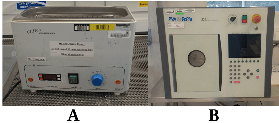
Figure 3.2: A) An ultrasonic bath used during solvent cleaning stages, and B) The Tepla Plasma Asher used during plasma cleaning and activation
