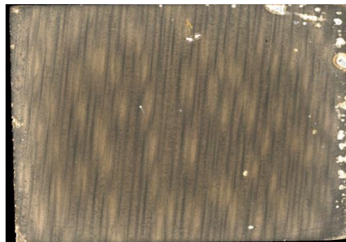
Figure 4.14: Optical Microscope and SEM BSE mode images showing the oxidation surfaces of CMSX-4 samples ( (001) planes ) exposed isothermally for various times at 550°C .
