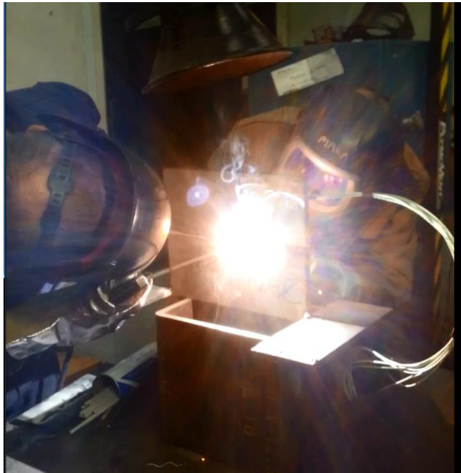
Figure 6.4: MMA welding simultaneously on each side of the plate
