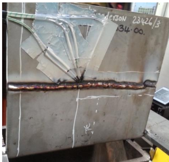
Figure 6.31: Bead-on-plate after welding
