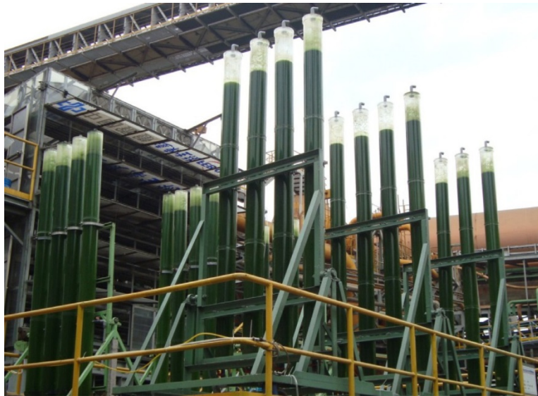
Figure 3.12. 3m long carbonation bubble columns with a total volume of 50 L each (Kao et al., 2014).
