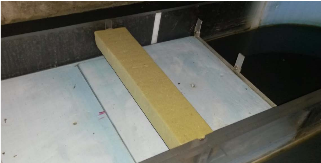
Figure 5.10. The wave diffuser. Note the grooves cut into the channel wall to hold the diffuser in place.
