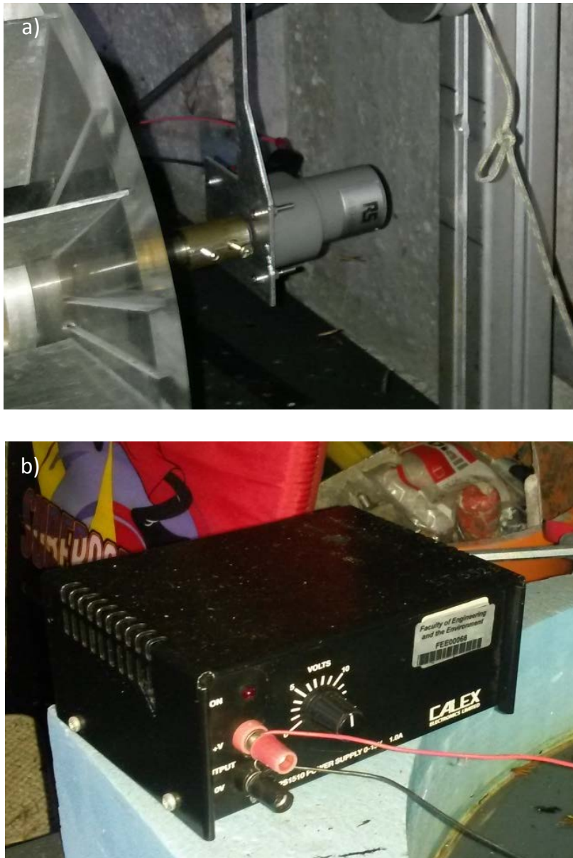
Figure 5.12. a) The motor used in the experiment with the direct transfer sleeve and b) the adjustable voltage regulator.
