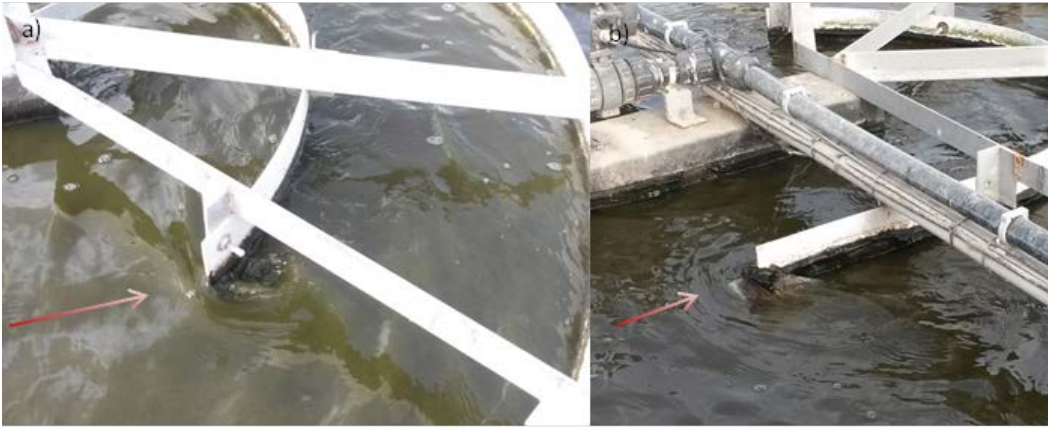
Figure 3.6. a) Wrongly positioned deflector. b) End deflectors with debris caught at the start causing a bow wave in front of the deflector. Both deflectors are part of a 20m 2 raceway on the FP7 ALL-GAS demonstration site located in Chiclana de la Frontera, Spain. The red lines indicate the direction of fluid flow.
