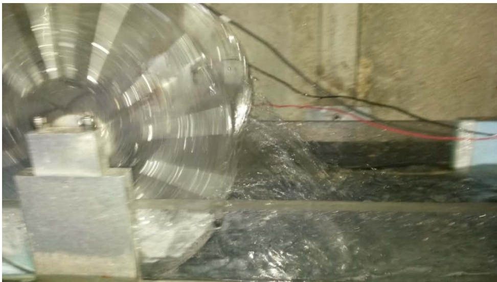
Figure 5.20. An image of the paddlewheel at a model wheel rotational speed of 30 rpm (13.4 rpm full scale). Notice the large extent of water lifting that occurs from the surface of the fluid.
