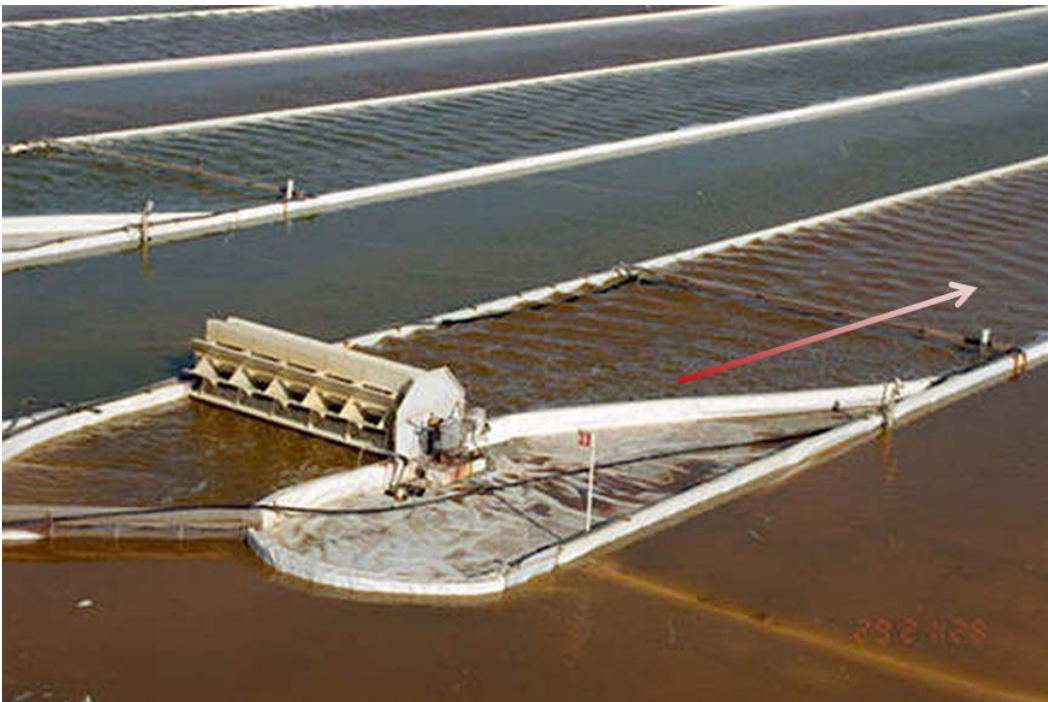
Figure 3.7. Asymmetric island bend design in use in a large-scale algal pond system (Tribal Energy and Environmental Information Clearinghouse, 2016). The red arrow indicates the motion of the fluid.
