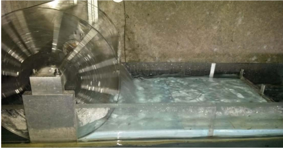
Figure 5.29. An image of the paddlewheel at a model wheel rotational speed of 30 rpm (13.4 rpm full scale) with the insert present.
