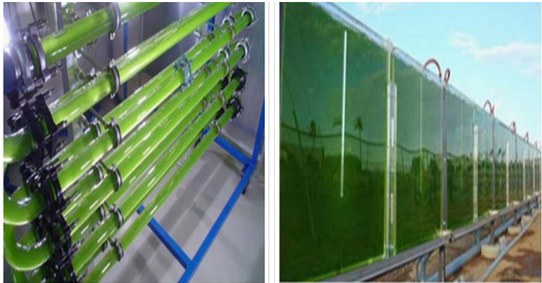
Figure 2.1. Photographs of two different types of photobioreactors. a) Horizontal tubular reactor. b) Flat plate reactor (Bitog et al., 2011).
