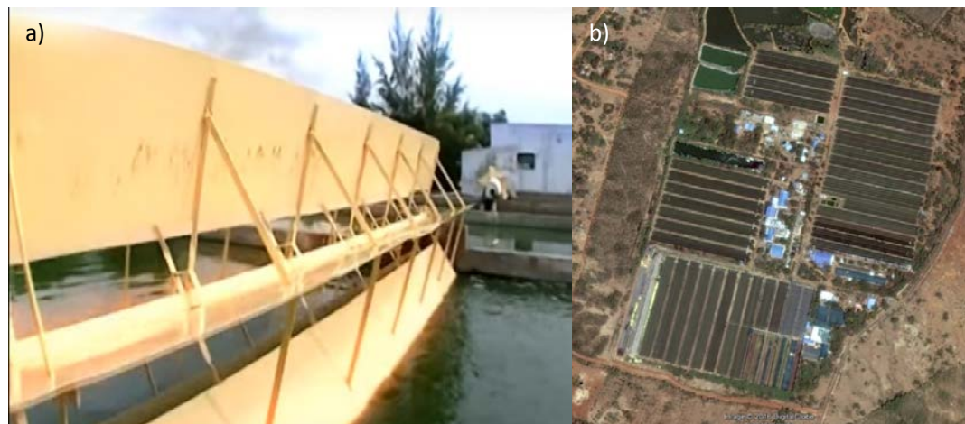
Figure 6.5. a) Parry Nutraceuticals paddlewheel system (Parry Nutraceuticals, 2011). b) Satellite image of the Parry Nutraceuticals production facility (Google Earth, 2016b).
