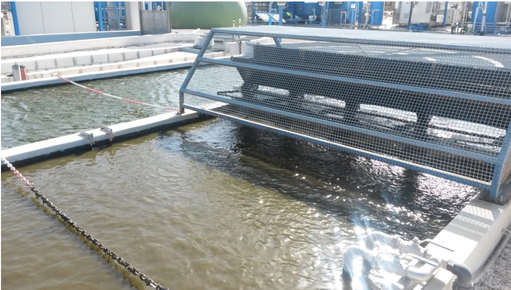
Figure 5.39. The fluid in the raceway was driven by a 1 m diameter flat 8-blade paddlewheel.
