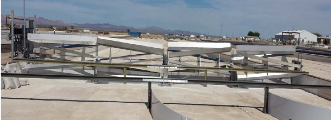
Figure 3.24. Large-scale 6-blade angled wheel in a full size raceway (Commercial Algae Professionals, 2015a).
