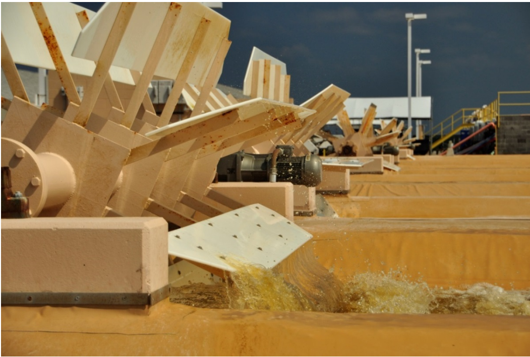
Figure 3.16. Standard flat 8-blade paddlewheel design (Cellana Inc., 2015). Notice the fluid lifted from the surface of the raceway falling away from the blade.
