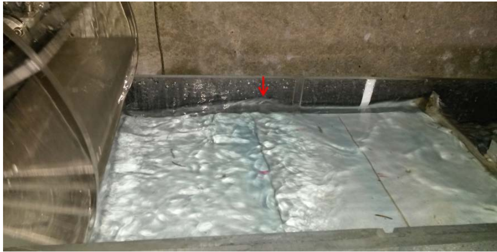
Figure 5.28. An image of the paddlewheel at a model wheel rotational speed of 10 rpm (4.5 rpm full scale) with the insert present.
