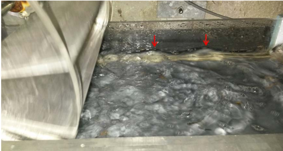
Figure 5.19. An image of the paddlewheel at a model wheel rotational speed of 10 rpm (4.5 rpm full scale). Notice the large standing waves indicated on the image.
