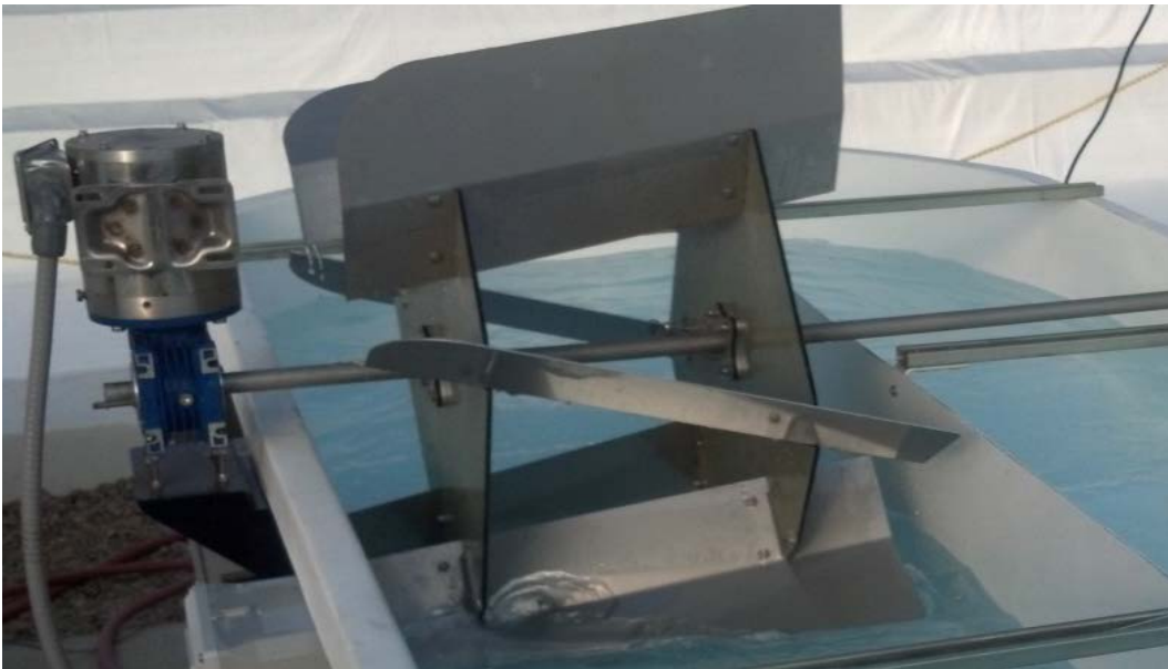
Figure 3.23. Experimental 6-blade angled wheel in a small inoculation pond (Commercial Algae Professionals, 2015b).
