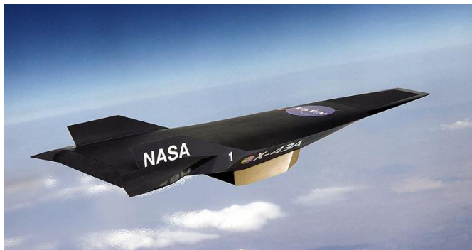
Figure 2.3. The X-43 hypersonic aircraft (NASA graphic).
