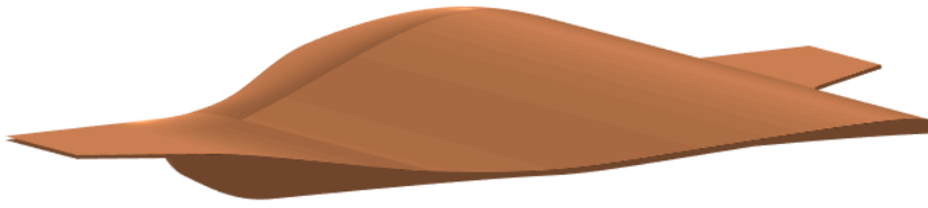
Figure 5.17. Simplified waverider-based aircraft geometry.
