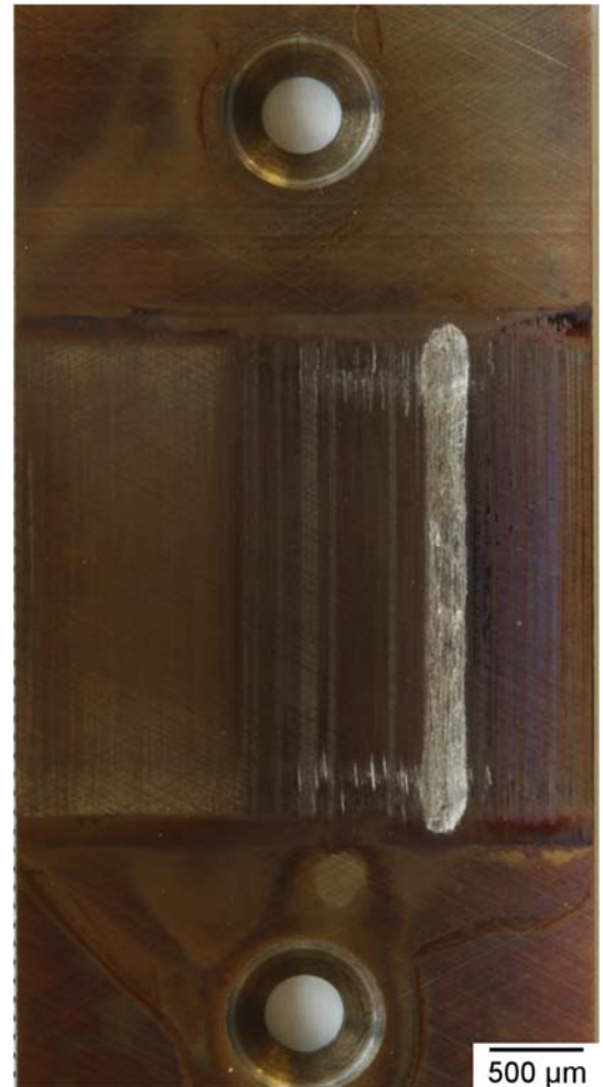
Figure 6.13: Optical images of the RLS1 cast iron wear scar.
