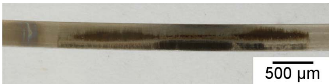
Figure 12.2: Optical images of the RLMS1 and piston ring wear scar.
