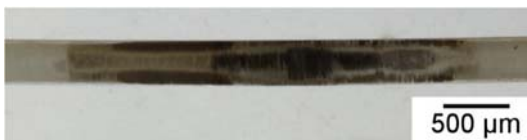
Figure 6.14: Optical image of the RLS2 piston ring wear scar.
