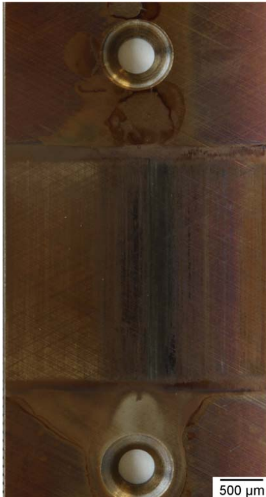
Figure 6.12: Optical images of the RLS2 cast iron wear scar.
