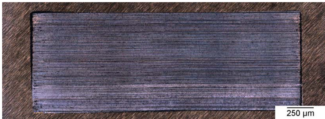
Figure 5.25: Optical image of intermediate scuffed nodular cast iron surfaces NIS1.
