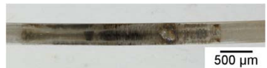
Figure 6.15: Optical image of the RLS1 piston ring wear scar.
