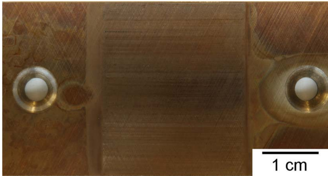
Figure 12.1: Optical images of the RLMS1 cast iron wear scar.
